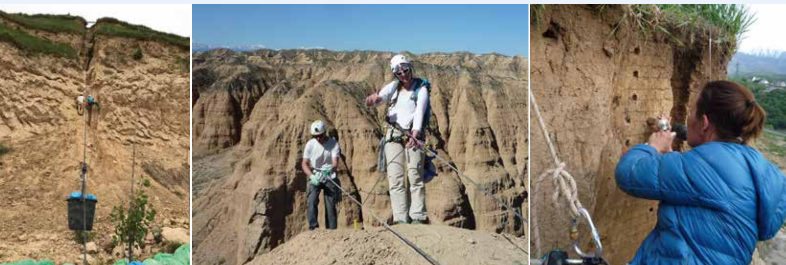
Figure 1: Impressions of fieldwork in Kazakhstan (L-R): continuous sampling by abseil at Remizovka; Group members probe 80 m of climate archives at Charyn Canyon; luminescence dating samples are collected in light-proof steel tubes at Remizovka (Credits: Charlotte Prud'homme).
