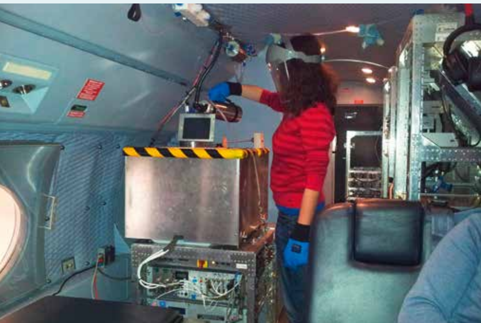
Figure 1: TRIHOP is an Instrument that measured \text{H}_2\text{O}_2 and total hydroperoxides, as well as \text{CO} , \text{HCHO} and \text{CH}_4 on board the High Altitude Long Operation (HALO) aircraft during the 2015 Oxidation Mechanism Observations (OMO) mission. TRIHOP stands for the combination of the instruments TRISTAR (Tracer In-Situ Tdlas for Atmospheric Research) and HyPHOP (Hydrogen Peroxide and Higher Organic Peroxides) (Credit: Uwe Parchatka).
