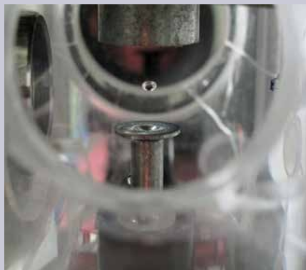
Figure 1: A free floating 2 mm water droplet in the ultrasound wave field of the Mainz Acoustic Levitator. Credit: Amelie Mayer, JGU.
