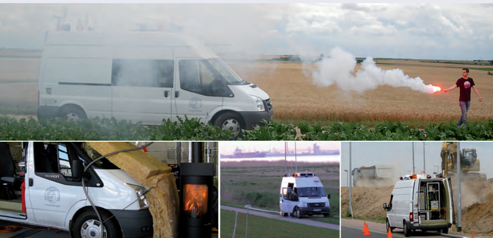
Figure 1: Measurement of emissions from “exotic” particle sources: Bengal fires, logwood combustion, sea-going ships, construction work. Photos: von der Weiden-Reinmüller, Freutel, Drewnick, Faber.
