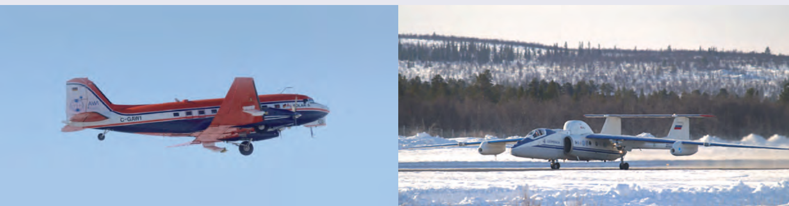
Figure 1: The research aircrafts: Left: Basler BT-67 modified DC-3 “Polar 5” of the Alfred-Wegener-Institut Helmholtz-Zentrum für Polar- und Meeresforschung during VERDI. Right: MDB high altitude aircraft M-55 Geophysica (ceiling of 21 km) during RECONCILE.
