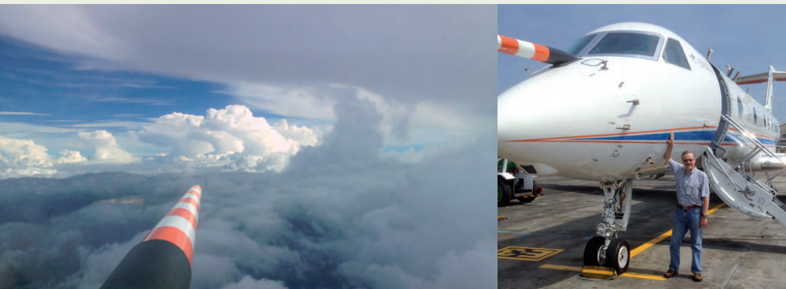
Figure 1: From the cockpit of the research aircraft HALO (right picture) one can see a special probe for air flow measurements aiming at the clouds.
