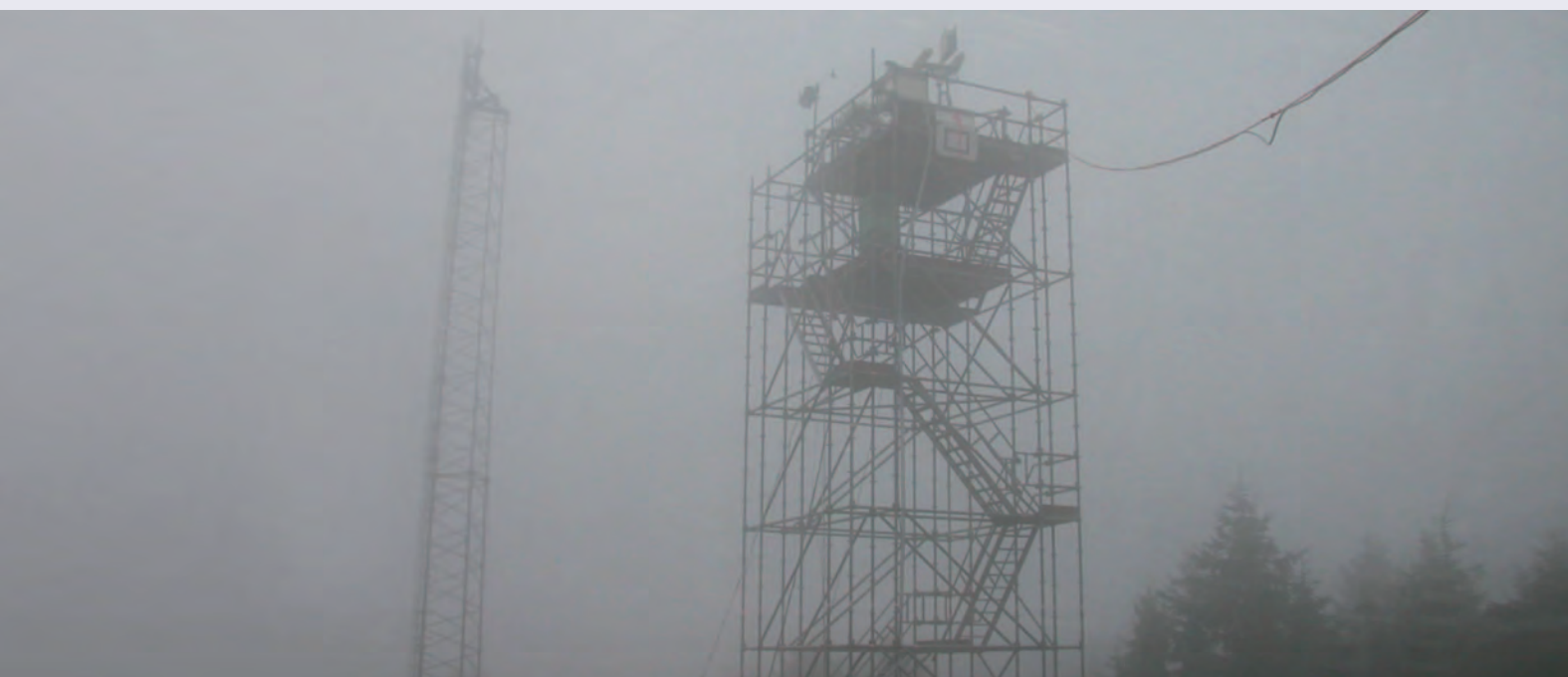
Figure 1: Cloud measurements: The picture shows the tower at the HCCT2010 field site "Schmücke". On the tower several instruments were installed to collect cloud water and to measure cloud droplet size distributions.
