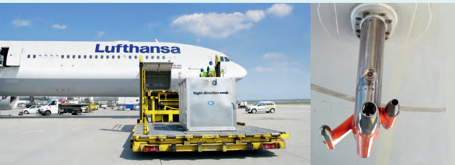
Figure 1: The 1.5 ton measurement container is loaded into the cargo bay of an Airbus 340-600 for 4 consecutive regular passenger flights. The inlet system visible in front of the belly fairing is a permanent part of this aircraft.
