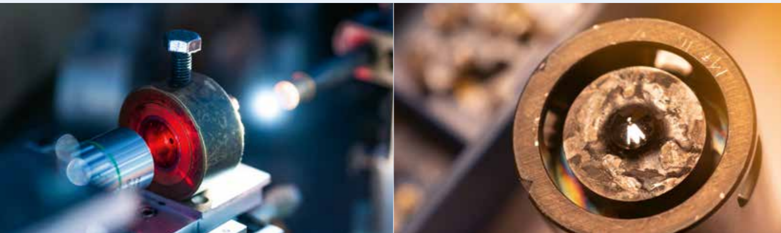
Figure 1: In a diamond anvil cell, more than one million bars can be created between two conical cut diamonds, with hydrogen rich materials such as hydrogen sulfide or yttrium hydride becoming superconducting at relatively high temperatures.
