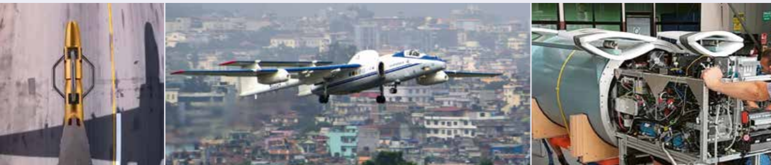
Figure 1: Left panel: ERICA sampling inlet during takeoff. Middle panel: Takeoff of the M-55 Geophysica from Kathmandu, 31/7/2017. Right panel: Integration of ERICA (inside a pressurized barrel) into the aircraft.
