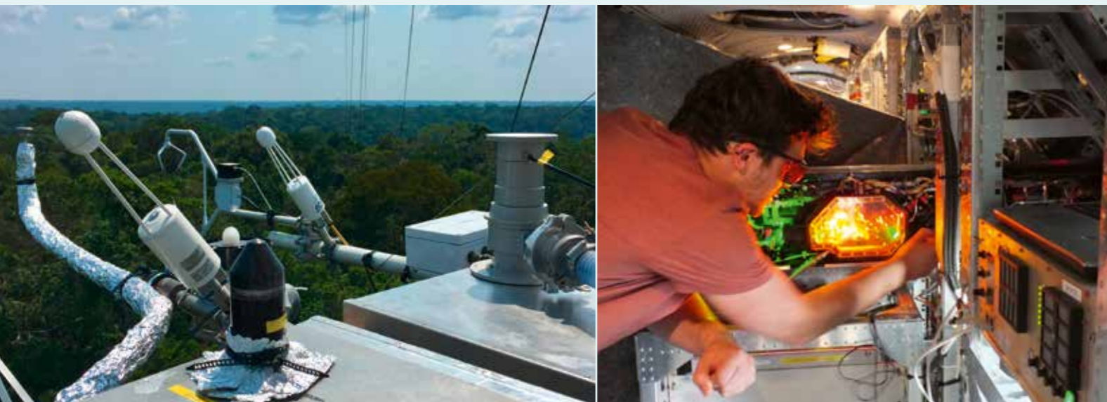
Figure 1: OH and HO 2 measurements above the canopy in Brazil (left), calibrating the OH and HO 2 measuring device onboard the HALO research aircraft (right).
